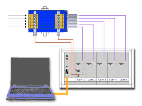
Fig. 2: CEM-array with negative high voltage
