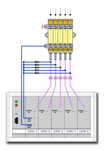
Fig. 3: CEM-array with positive high voltage
